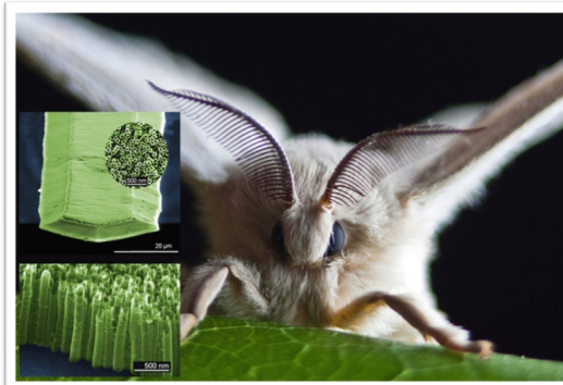
Silk moth antennas (depicted in large photo) are unique in nature and according to experts this can be imitated can utilizing micromechanical sensors with optical signal detection to detect low levels of explosives. Smaller photos illustrate Silicon micro cantilevers modified with a three-dimensional layer of vertical titanium dioxide nanotubes.
