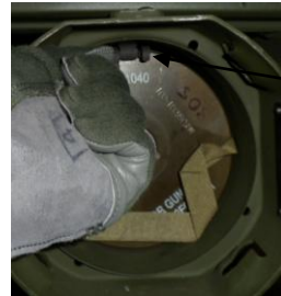
Single loop held in the up position to ensure it is fully extended over the top of the case base lip
