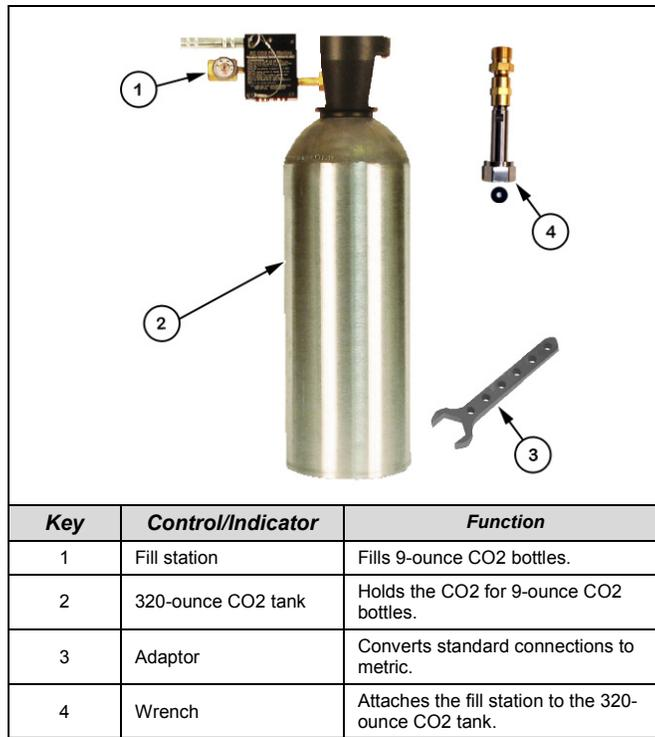
Figure 17. NPSSD fill station
