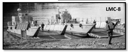
in each of two sections. LCM-8s (also known as "mike boats") can transport cargo, troops, and vehicles from ship to shore or in retrograde movements. It is also utilized in harbor lighterage and utility work where its small size and shallow draft (4 ft. 6 in.) allow its use in confined areas. It's designed for use in rough or exposed waters and is capable of operating through breakers and grounding on a beach. The bow ramp permits RO/RO operations with wheeled and tracked vehicles.
