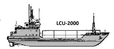
The company consists of two platoons, each with an with an LCU-2000 capable of moving 400 Soldiers, five M1A1 battle tanks, 250 short tons of cargo, 24 20-foot containers per lift.
