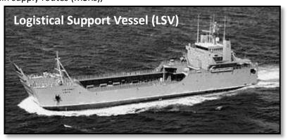
The cargo deck is designed to handle any vehicle in the Army inventory and can carry up to 15 M1 Abrams main battle tanks, 82 ISO standard containers, or 2,000 short tons of unit equipment/supplies per lift – the equivalent payload of 40 C-17s.
