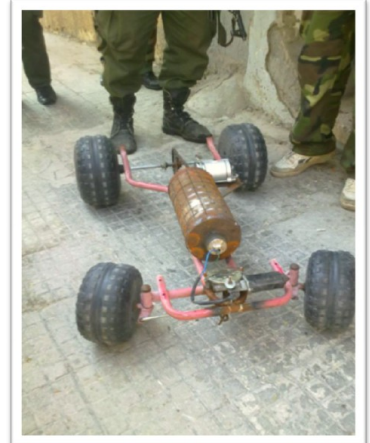
Assad Regime published photo of an IED mounted atop a pedal go kart, claiming it could be piloted and detonated remotely. Much like the device used by the Free Syrian Army (FSA) on the 10 th of June in an attack targeting a military roadblock in Damascus.
