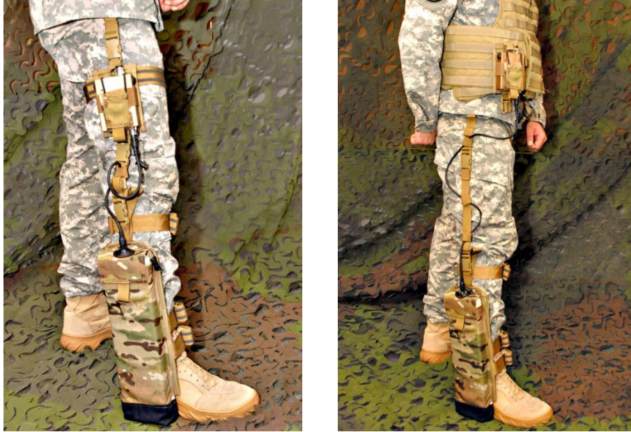
Figure 2: Strider Detector System in operational configuration, with the Control Unit mounted on the thigh (Left) and with the Control Unit mounted on the vest/IOTV (Right).
