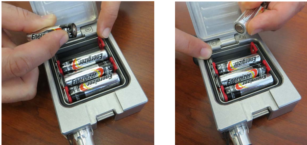
Figure 3: Inserting four AA batteries into Control Unit, aligning Positive battery terminals with Red battery slot terminals (left) and aligning Negative battery terminals with Black battery slot terminals (right).
