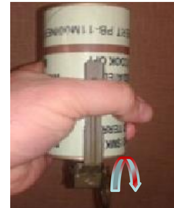
Left Hand Grip: Rotate pull ring clockwise (away from the body) to disengage Confidence Clip
