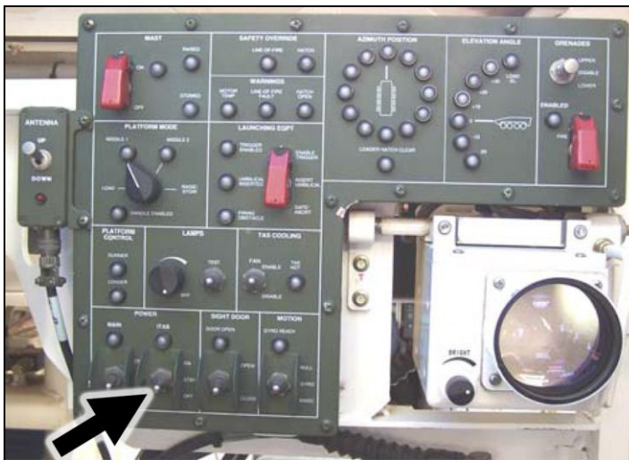
Figure 3-1. TAS power switch on ATGMV gunner's control panel.
