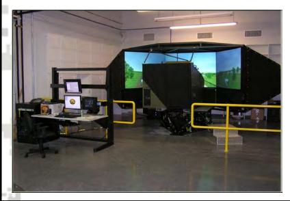
•Purpose/Contribution: The device consists of a simulated vehicle cab, instructor/operator station, a visual system, a 6-DOF motion system, AAR station and a computational system. Common Driver Trainer/Stryker will be the baseline of a Common Driver Trainer architecture consisting of a Stryker, Tank, and MRAP version. The Stryker Driver Trainer provides initial and sustainment driver training at training institutions and operational installations.
