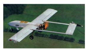
The Shadow UAV is the Brigade Commander's primary Reconnaissance, Surveillance, and Target Acquisition (RSTA) asset. The Shadow is equipped with an Electro-Optical and Infrared camera (EO/IR). It has a range of 50 km and can fly for up to five hours and altitudes up to 15,000 ft.
