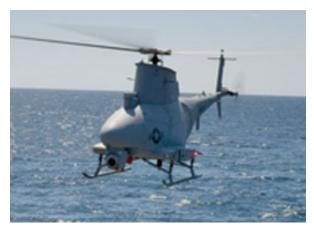
The Fire Scout is a Vertical Take-Off and Landing Tactical Unmanned Aerial Vehicle (VTUAV) system and is comprised of up to three MQ-8B Fire Scout air vehicles, ground control stations, and associated control handling and support equipment. The VTUAV system will provide a significant improvement to organic surveillance capability. With vehicle endurance greater than eight hours, a VTUAV system will be
