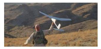
The Raven UAV is small and can be transported easily in three small cases that fit into a ruck sack. The crew can bring it with them and operate wherever the unit goes, contingent on ROZ and A2C2 approval. The Raven has three different cameras that attach to the nose of the plane: an electrical optical
