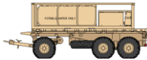
M1076 TRAILER PLS 8X20 W/LOAD HANDLING SYSTEM 2000GAL CAP WATER TANK (HIPPO)
