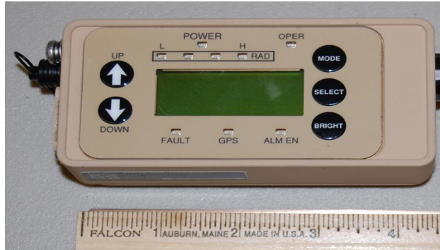
RCU Front Panel Showing Indicators
