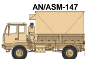
ELECTRONICS SHOP SHELTER MOUNTED AVIONICS: AN/ASM-147 (SHOWN MTD ON M1078 LMTV) (H01912)
