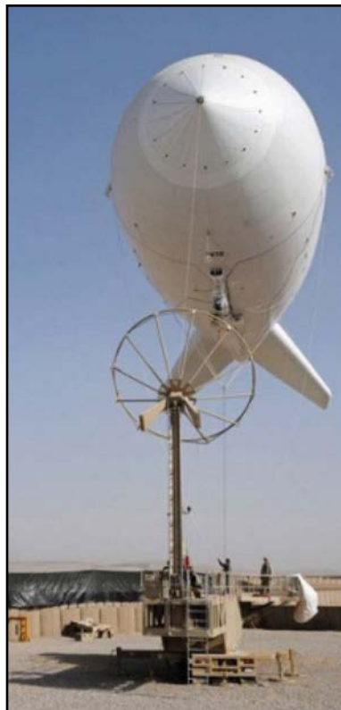
Figure 1-5. The PTDS is tethered with multi-mission sensors.
