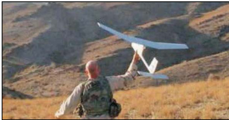
Figure 1-1. Raven, small, portable, short-range unmanned aircraft system.
