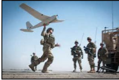
Figure 1-2. PUMA, small, portable, long-range UAS.
