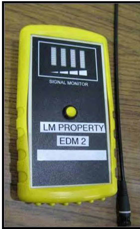
Figure C-5 Field Test Set
