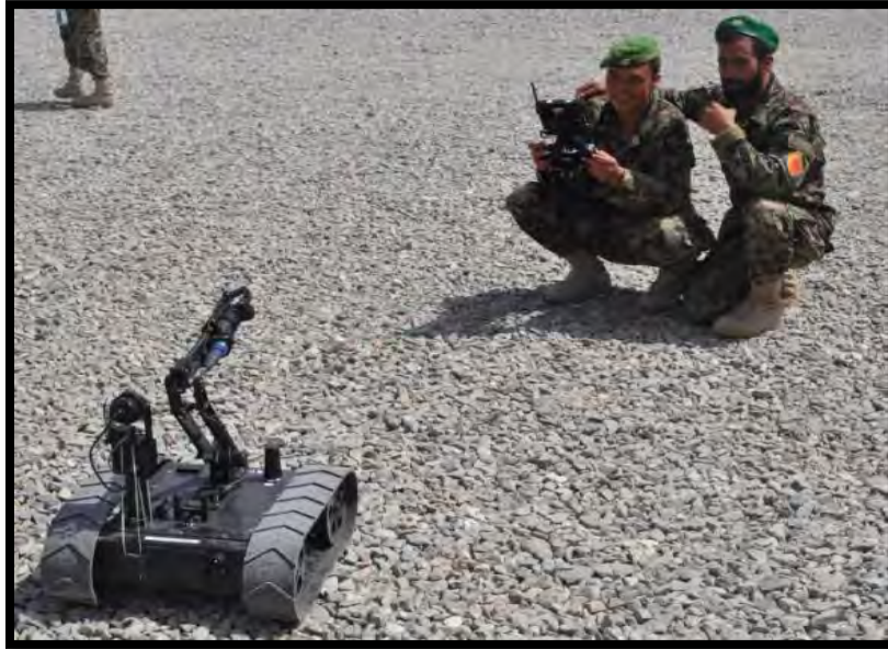
Figure 2-24 MMP 30 EOD Robot
