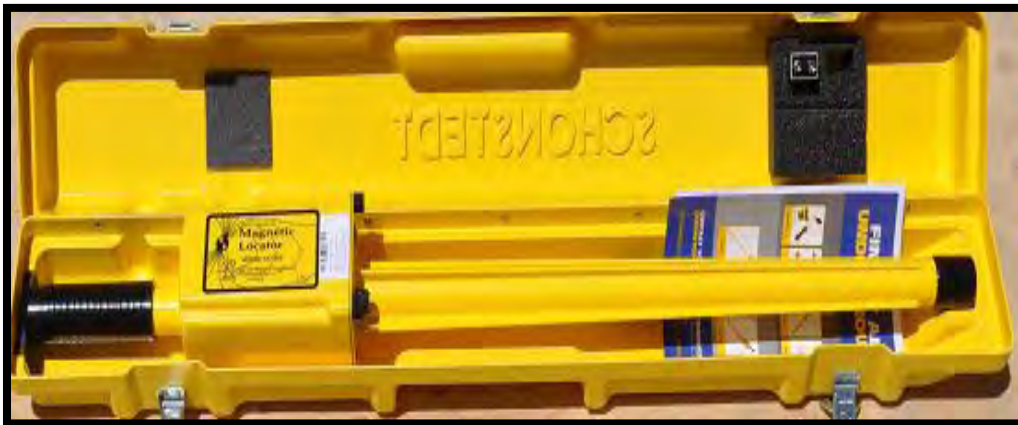
Figure 2-31 Schonstedt Magnetic Locator
