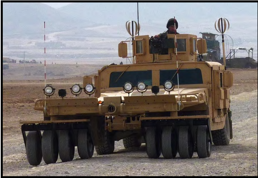
Figure 1-3 Panama City Mine Roller Mounted on an M1151 HMMWV
