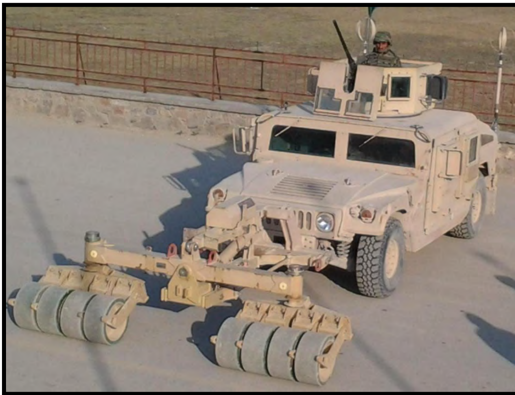
Figure 1-4 SPARK OIF Track Width Roller Mounted on an M1151 HMMWV
