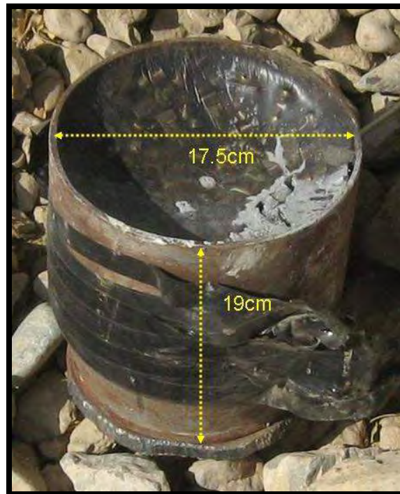
Figure 3-24 Example of a Directional Fragmentation Charge
