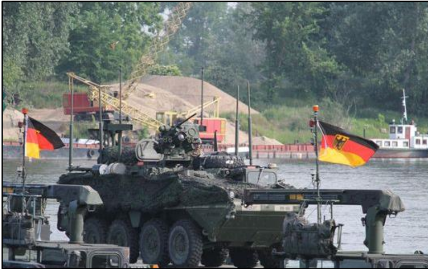
Figure 12. A US Stryker crosses the Vistula River on a bridge made of German and British M3 amphibious rigs
