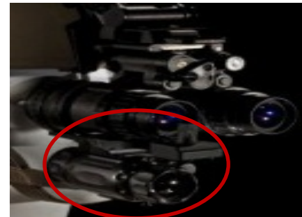
COTI (Clip-On Thermal Image) capable – thermal overlay on NVG
