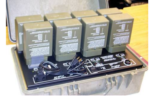
Charger and batteries (BB2847 rechargeable)
