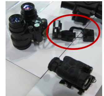
COTI (Clip-On Thermal Image) capable – thermal overlay on NVG
