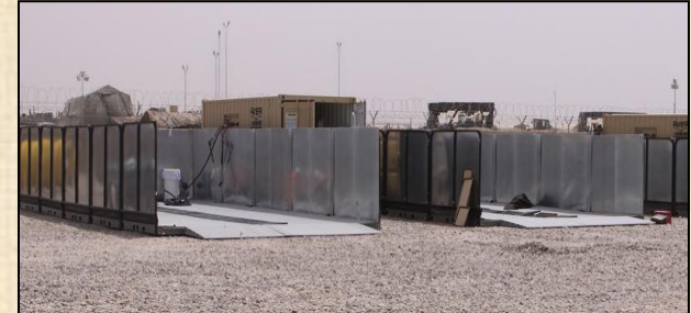
Pictured above is one double lane mobile wash rack 18' x 42' and 20' container completely setup.
