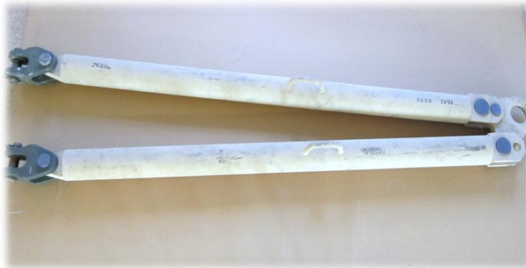
U.S MARINE CORPS MEDIUM DUTY TOW BAR NSN: 2540-01-496-8356 WEIGHT: 226 LBS. LENGTH WITHOUT ADAPTER: 60 IN CAPACITY: 83,000 LBS END ITEM: MTRV MK36
