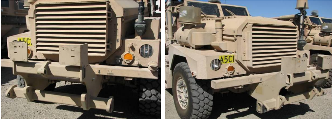
SPARK Interface Bracket on the FPI Cougar 4x4 and 6x6 MRAP Vehicle.
