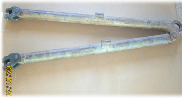
U.S ARMY HEAVY DUTY TOW BAR NSN: 2540-01-434-8595 WEIGHT: 282 LBS. LENGTH WITHOUT ADAPTER: 88 IN CAPACITY: 139,000 LBS (Weight of M88A2) END ITEM: M88A2 (HEMTT AAL)
