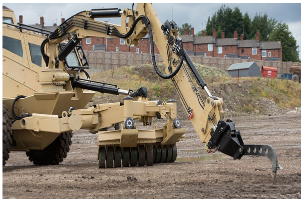
PEROCC incorporates the remote arm to Interrogate a suspected device
