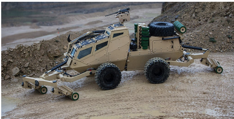
PEROCC with full compliment of attachments to include a CROW mounted weapon system
