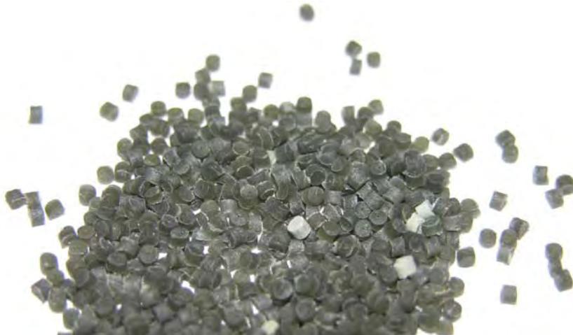
Close-up of M45 Propellant. Note the light and dark color gray cylinders present.
