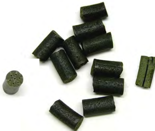
Top of grain shown on left; split grain showing green interior on right
