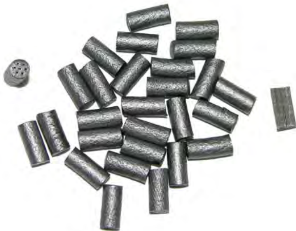
Top of grain shown left; split grain showing gray interior on right
