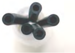
Top view of M7 sticks depicting large single perforation
