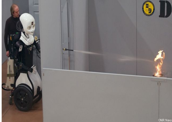
A prototype robot incorporating SiN-VAPOR sensors to detect and fight fires.
