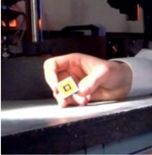
SiN-VAPOR sensor utilizes nanowires
