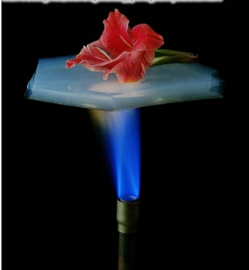
A flower is on a piece of aerogel which is suspended over a Bunsen burner. Aerogel has excellent insulating properties, and the flower is protected from the flame. Source: NASA JPL, "Aerogel flower," Wikimedia Commons, retouched by Wikimedia Commons user JovanCormac, 23 October 2007, https://commons.wikimedia.org/wiki/File:Aerogelflower.jpg . Image is in public domain.
