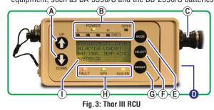
(A) UP/DOWN – Scroll display up (F) SELECT – Button selects display line. (B) Indicator LEDs – POWER, **G** BRIGHT button
