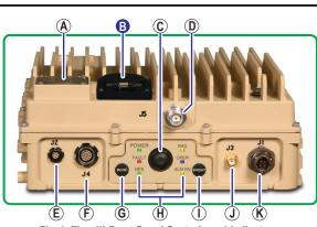
Fig. 1: Thor III Front Panel Controls and Indicators
