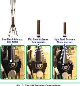
Fig. 2: Thor III Antenna Connections
