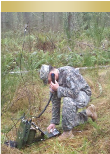
(Above) SGT Anthony Landis, Communications NCO for A/3-38 CAV, successfully transmits data and voice sky wave communications over 14 miles, from Merrill DZ to the A Troop Headquarters, using an AN/PRC-150 high frequency radio kit and a field expedient half-wavelength dipole NVIS antenna, elevated just 1 meter above the ground.
