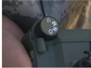
Figure 3-11. Mode Selector Switch in Off position.
