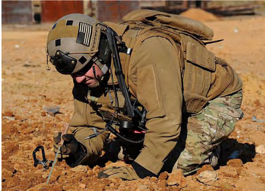
Figure 4-6. NSWC IHEODTD TSD. A platoon member uses a mine probe to ensure disturbed dirt around a blast crater is safe. (Photo Credit: USN)
