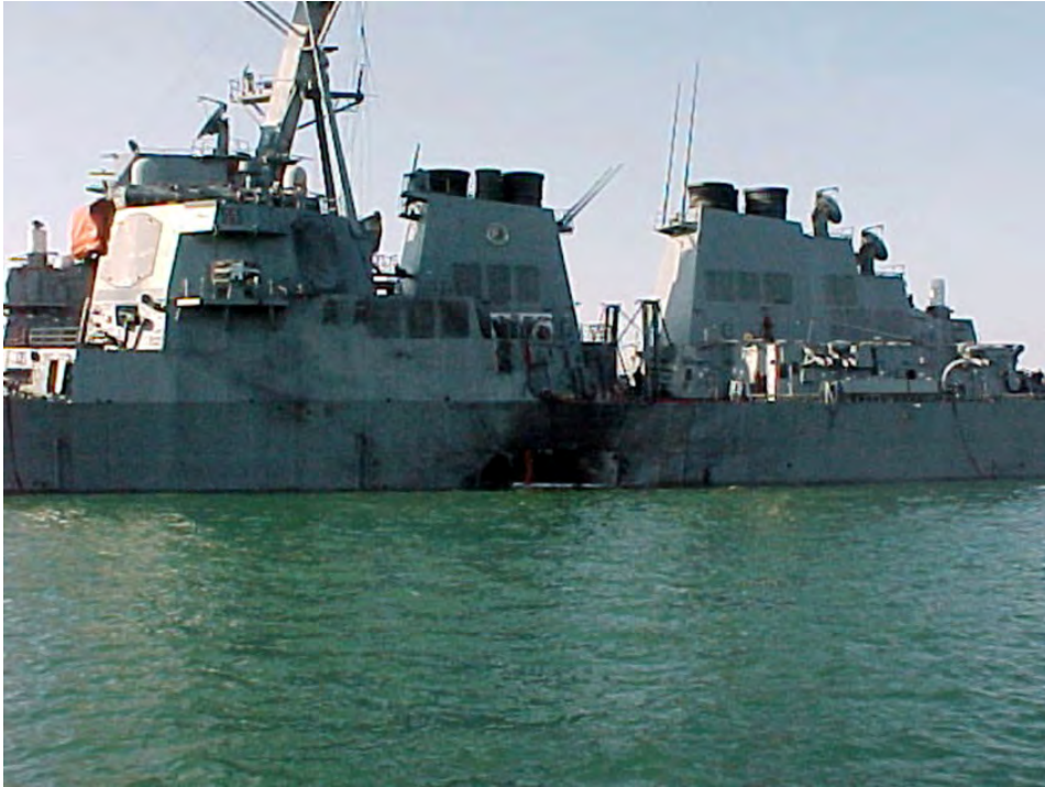
Figure 2-13. Vulnerable Target. The USS Cole (DDG-67) was damaged by a water borne IED while refueling in the Port of Aden, Yemen, October 12, 2000. (Photo Credit: USN)
