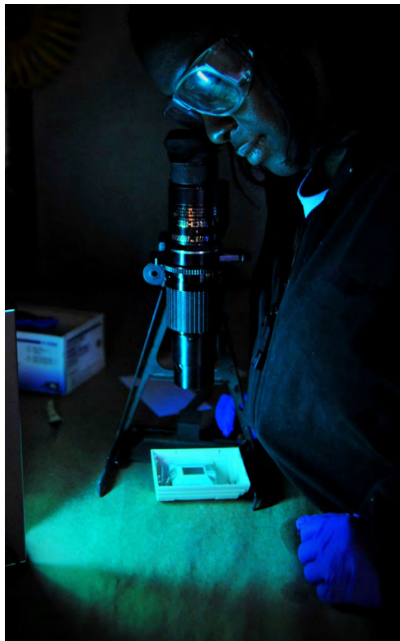
Figure 5-3. Latent Print Examination. Latent print examiner at a deployed exploitation laboratory uses a reflective ultraviolet imaging system to analyze fingerprints. (Photo Credit: USAF)
