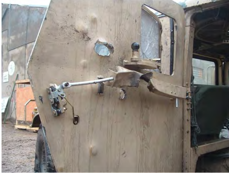
Figure 9-2. Battle Damage. This damage was caused by an anti-armor IED and documented for further analysis by CIAD. (Photo Credit: CJTF Troy)
