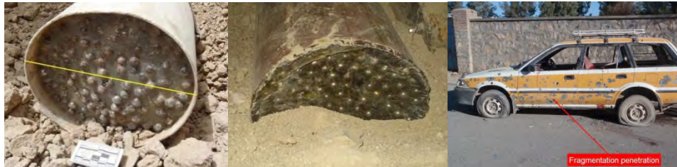
Figure 2-12. Pictures of Directional Fragmentation Charge, Directional Focused Fragmentation Charge, and Damage Caused (Photo Credit: CJTF Paladin)
