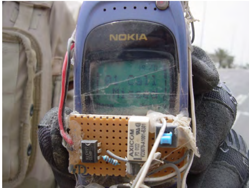
Cell Phone used as an IED Switch in Iraq (Photo Credit: DIA)
