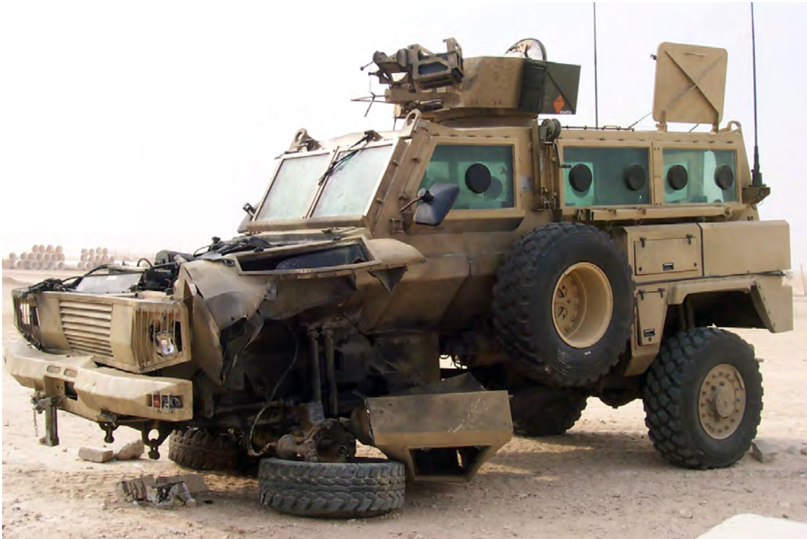
Figure 2-10. Underbelly Attack Results. This shows the outcome of an underbelly attack using an IED buried in the road or in a culvert. (Photo Credit: JIEDDO)
