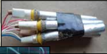
Christmas Tree Light Bulb - Improved Electric Blasting Cap - Somalia
