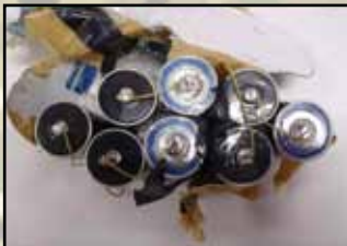
Batteries Taped / Connected Together or Wires Soldered to Terminals*
