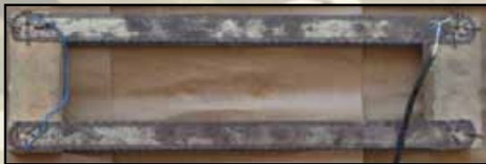
Four Hacksaw Blade Pressure Plate - Somalia
