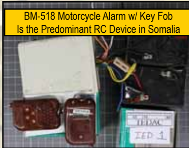
Complete Switch (BM-518 Motorcycle Alarm) w/ Dual 6v Batteries - Somalia
