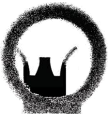
Incorrect Front sight misaligned left
