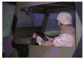
Using the USMC-ODS, initial driver trainees complete go/no go requirements of vehicle licensing before transitioning to actual vehicle driving, thereby reducing the costs of actual vehicle fuel and maintenance and actual vehicle usage. The USMC-ODS is not intended to replace training with the actual vehicle, but rather to complement it. Basic and advanced skills taught in the simulator are taught in the actual vehicle.
