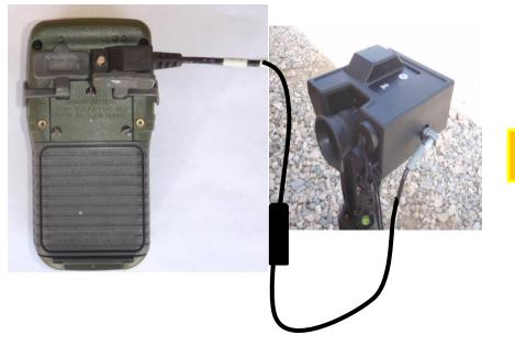
Connect the J2 Data Interface Connector on the DAGR to the RS170 interface plug on the PLRF-15C utilizing the adaptor cable with integrated trigger.
