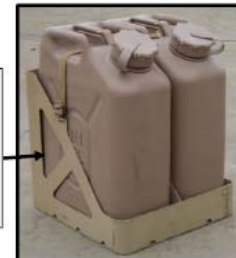
User suggests stowing the fuel cans on the exterior of the vehicle and away from the gear on the rear deck. A fuel can stowage bracket should be added to vehicle design. Field solution: Attach fuel can stowage bracket (NSN 5340-01-556-5767) to left rear corner of the antenna structure as shown.
