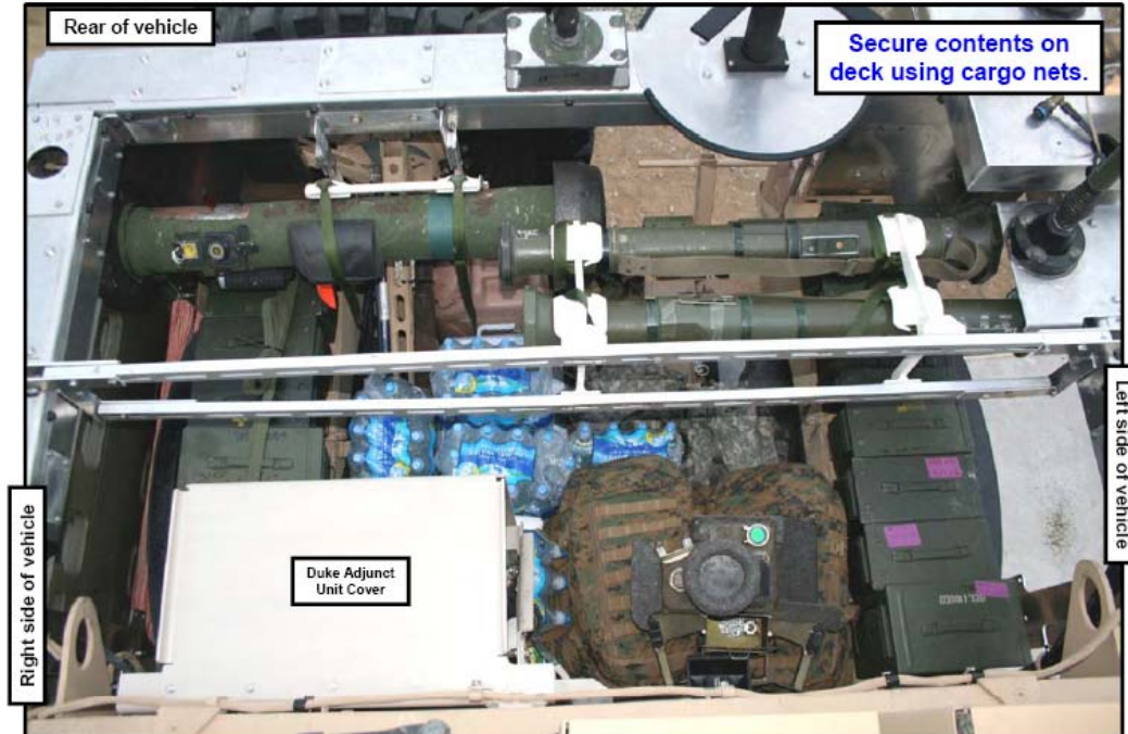
Stowage brackets for the Javelin and AT-4's should be added to vehicle design. Concept shown uses brackets from a Stryker vehicle and modified for the M-ATV. User recommends removing 1 of 2 Javelin missiles identified on the vehicle load list due to lack of stowage space. Javelin missiles are not carried by all vehicles; mission/role dependent.
