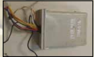
RC Receiver - BM-518 Motorcycle Alarm - Somalia
