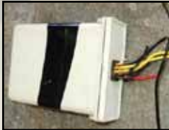
RC Receiver - BM-518 Motorcycle Alarm - Somalia
