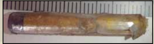
HME Filled Plastic Pen Body - Improvised Blasting Cap
