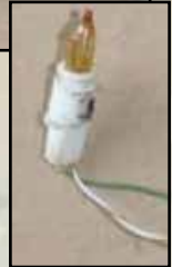
Christmas Tree Light Bulb - Improvised Electric Blasting Cap - Somalia
