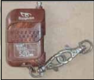
RC Transmitter – BM-518 Motorcycle Alarm Key Fob - Somalia
