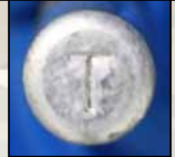
Electric Blasting Cap Ends - Somalia
