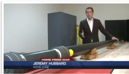
Jeremy Hubbard reports, Skydex utilizes a huge shock tube that mimics the effects of a huge IED blast, big enough to blow up a large military vehicle. The scaled-down blast simulations show them how well their product works, and what needs to be done to improve it. KDVR.com
