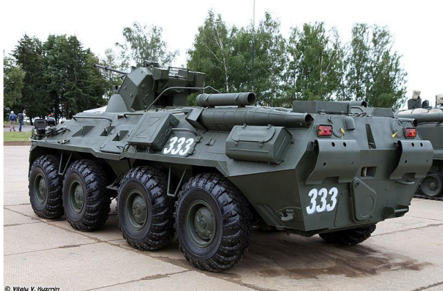
BTR-82A with good view of the stowed snorkel system
