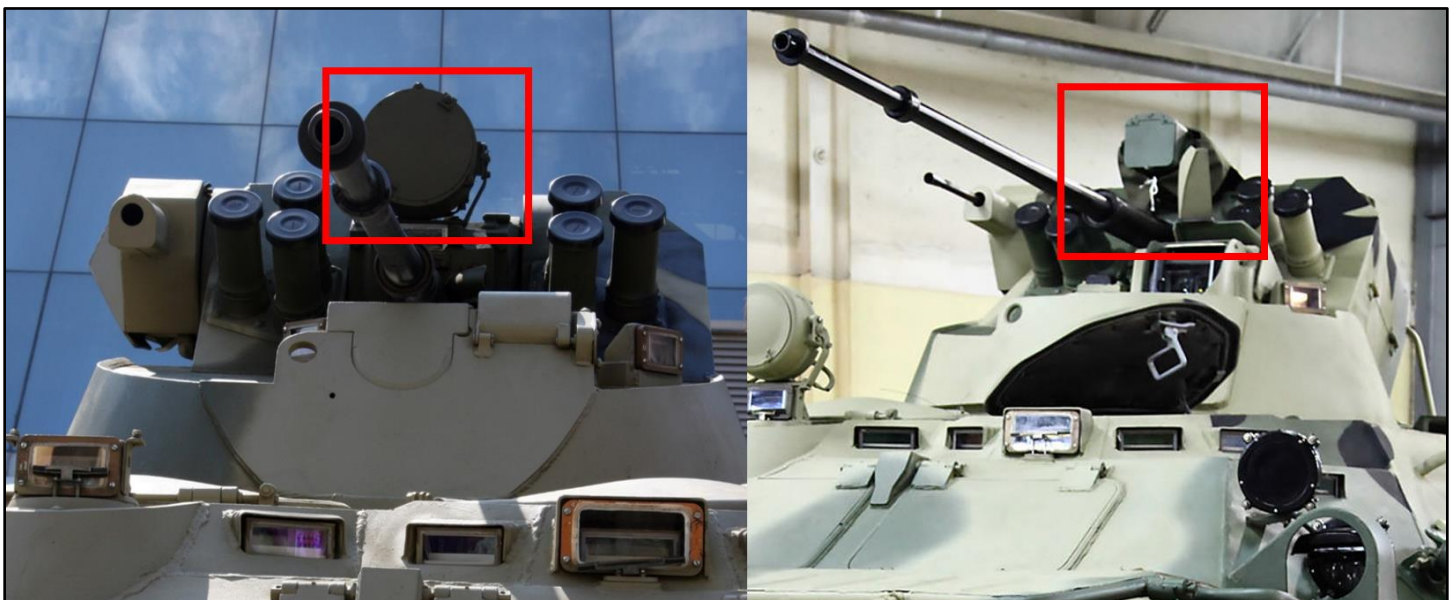
Figure 2. Comparison of the BTR-80 Laser Illuminator/IR Searchlight on the left to the BTR-82A on the right (photos by Vitaly V. Kuzmin)
