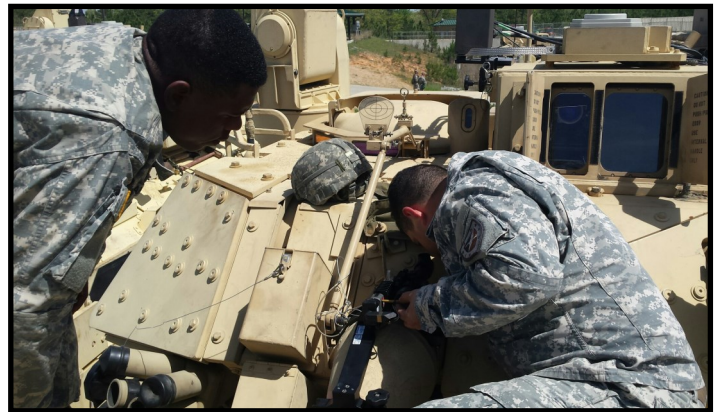
Two Soldiers align a laser on a Bradley Fighting Vehicle
