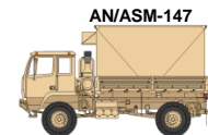
ELECTRONICS SHOP SHELTER MOUNTED AVIONICS: AN/ASM-147 (SHOWN MTD ON M1078 LMTV) (H01912)
