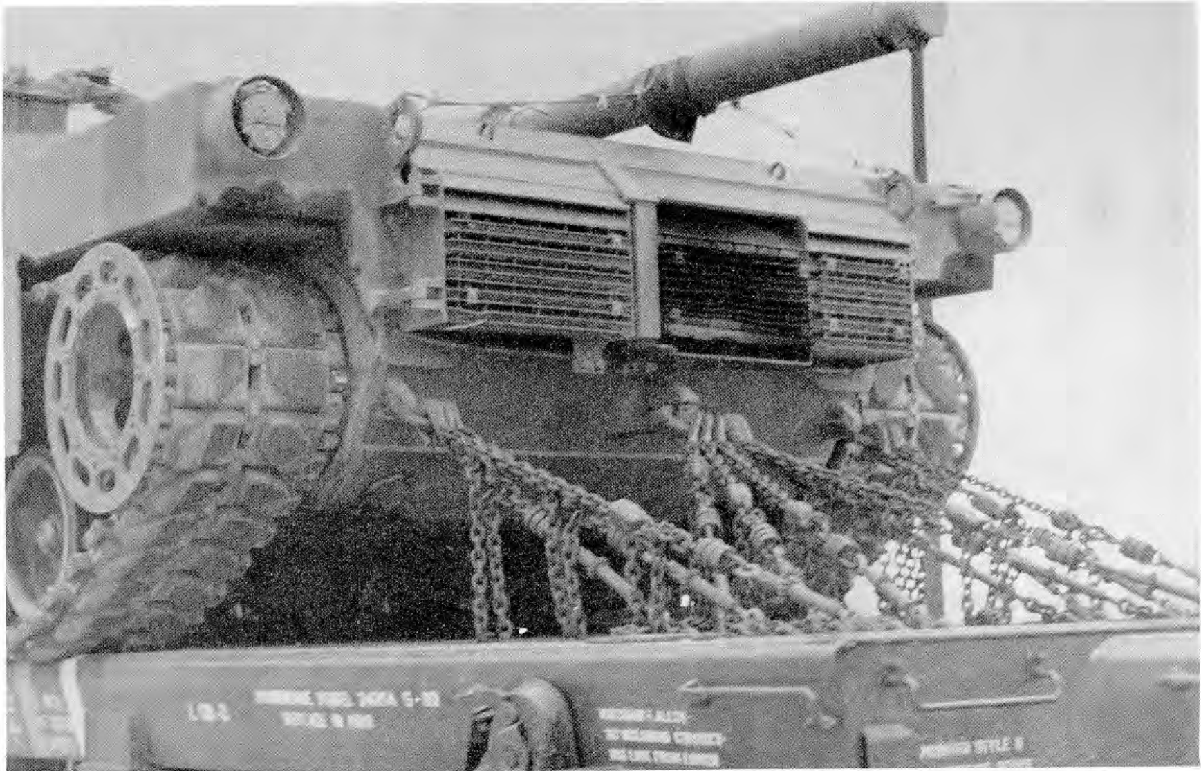
Figure 4-5. Rear view of M1 tank loaded and restrained on 140-ton DODX flatcar.
