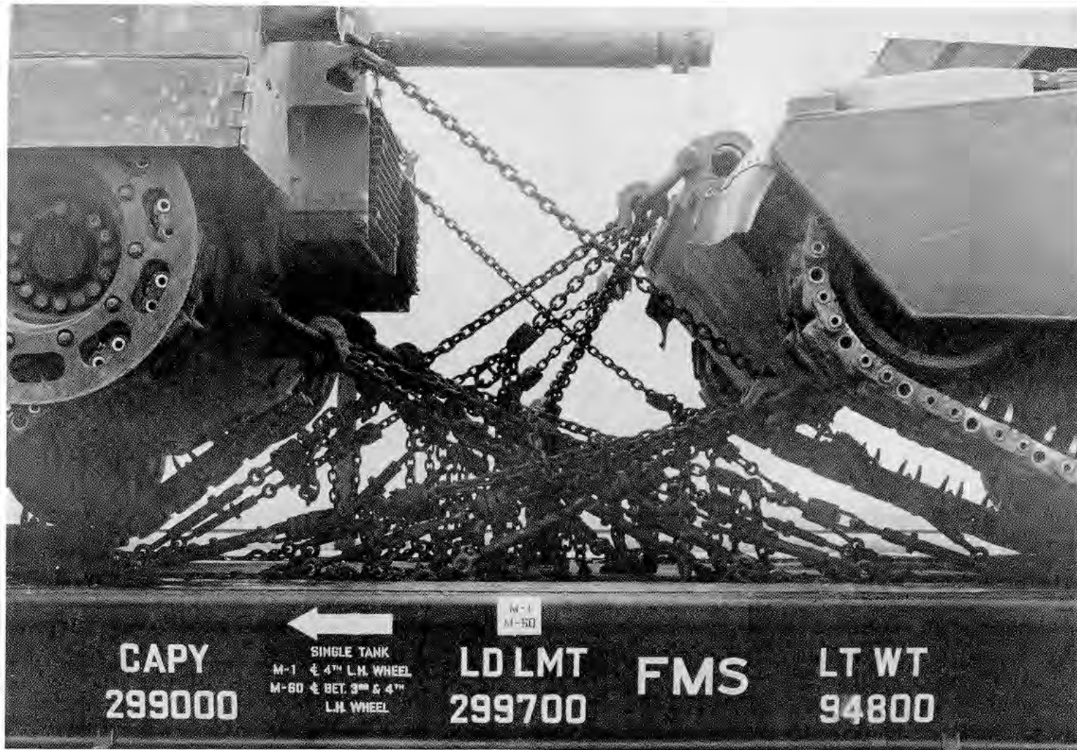
Figure 4-6. Between-tanks arrangement of chain tiedown devices.
