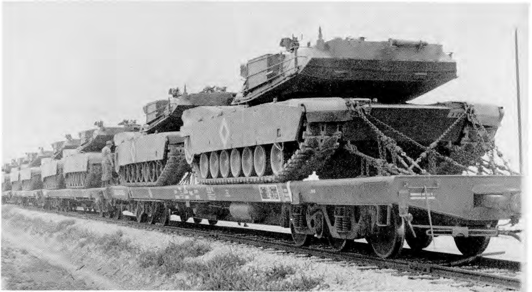
Figure 4-4. Front view of M1 tanks loaded and restrained on 140-ton DODX flatcar.
