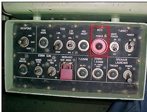
MCD light on Bradley System Control Box
