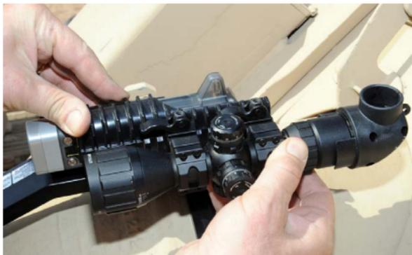
8. Install the right-angle prism on the alignment kit.
