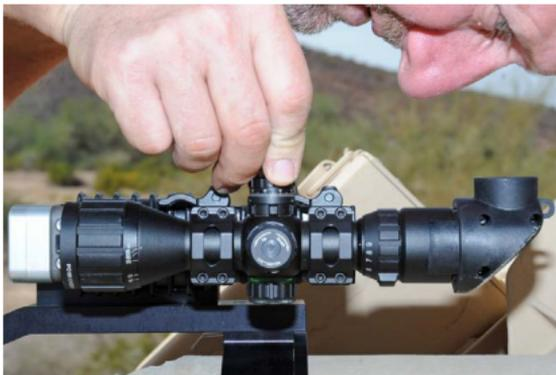
Adjust the alignment scope using the adjustment knobs on the alignment scope so the crosshair is on the 25 mm gun sight aiming point.
