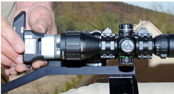
11. Rotate the SAAD optics in front of the alignment scope, into line of sight.
