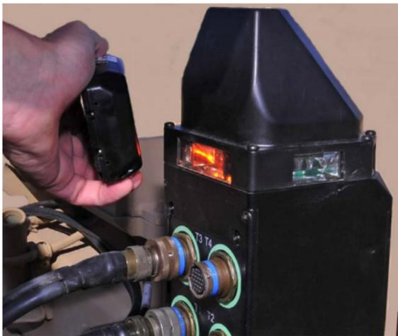
The IR sensor is located on the front of the CKM.
