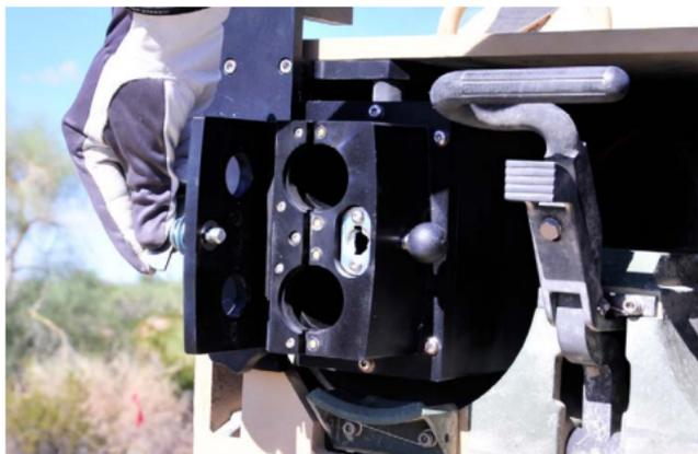
3. Visually check to see that the cartridge chambers are completely empty.
