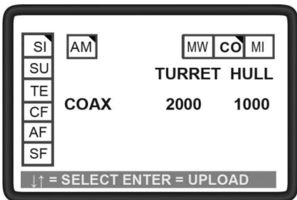
A preset upload time starts to count down. During the upload sequence a full ready box (turret) or remaining ammunition in hull is transferred.
