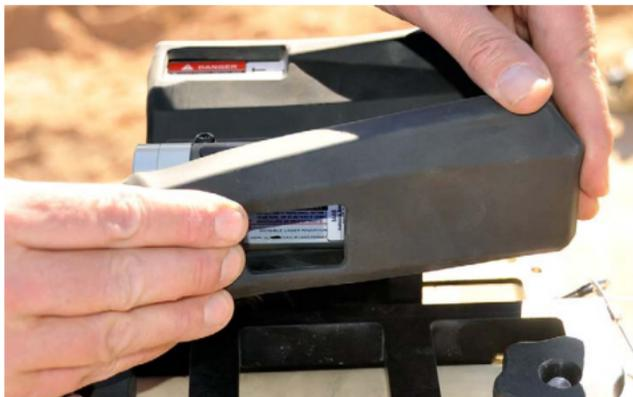
Starting at the back of the LT, fit the cover over the antenna and then slide the rubber cover over the front of the LT.
