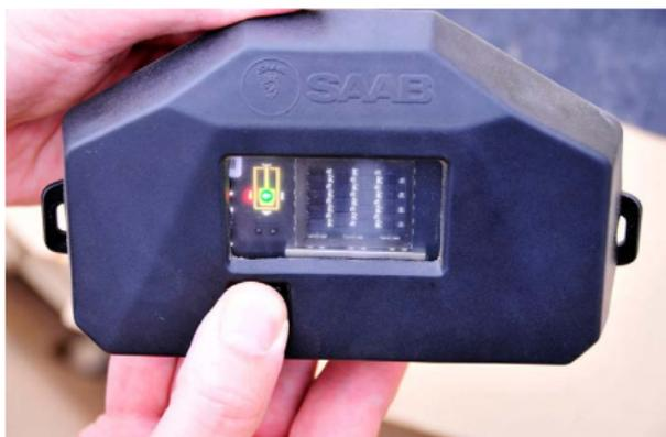
3. Hold the WDU window to the IR window on the TIM to establish IR communication.
