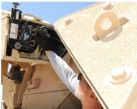
4. Visually check to see that the cartridge chambers are completely empty.
