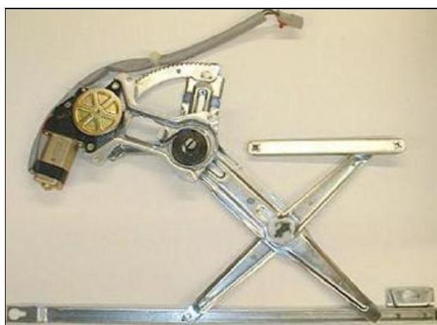
Car window regulator cannibalized for controlling the steering wheel
