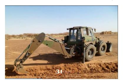
A French Sapper uses an excavator to build an anti-pickup obstacle for force protection.
