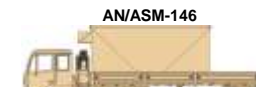
AN/ASM-146 ELECTRONICS SHOP SHELTER MOUNTED AVIONICS: AN/ASM-146 (SHOWN MTD ON M1085 MTV) (H01907)
