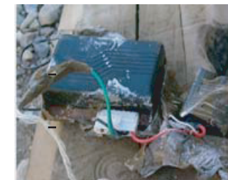
RC Unit from Car Alarm
