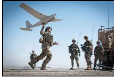
Figure 1-2. PUMA, small, portable, long-range UAS.
