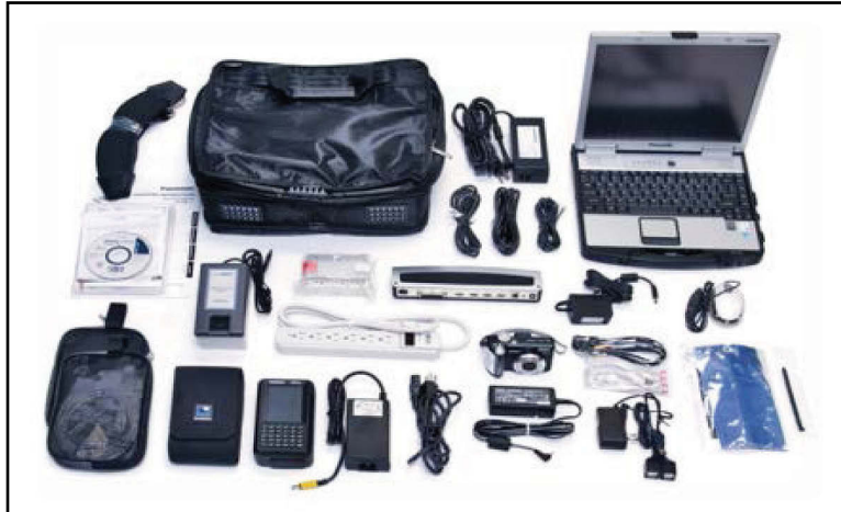
Figure 1-7. The BAT-A system that collect biometric characteristics on persons of interest.
