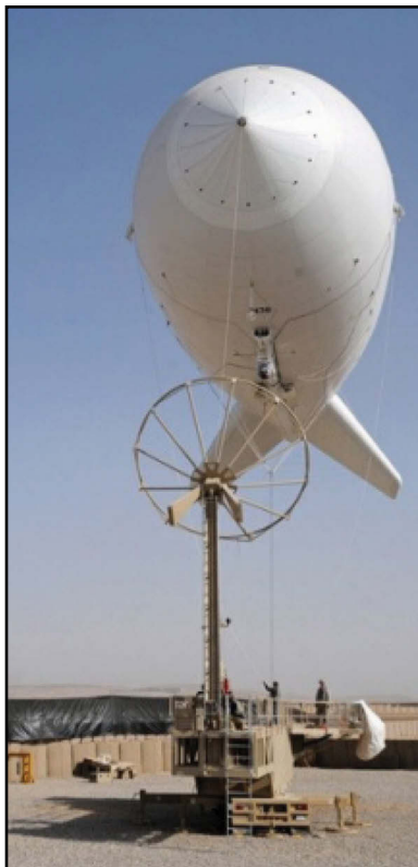
Figure 1-5. The PTDS is tethered with multi-mission sensors.
