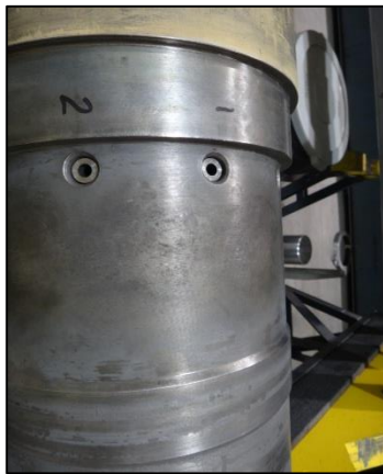
Figure 2. M284 Cannon bore evacuator holes and bushings.
