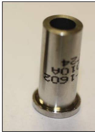
Figure 2. M284 Cannon bore evacuator holes and bushings.
