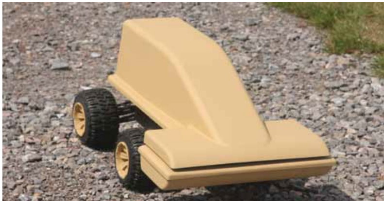
This system incorporates the same Ground penetrating technology that is used in the MINEHOUND
