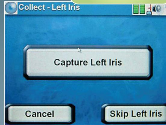
Keep the crosshairs centered on the iris and move in or out until the red bars appear. Focus distance is 12-14 inches. When the left bar is full, press and hold the trigger button. The focus bars will turn green. When you have a good iris image, touch the "Accept" button.
