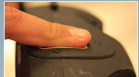
The curved tip area of the finger is not pressed against the capture area. Flat portions of the finger are placed on the flat portions of the capture area.
