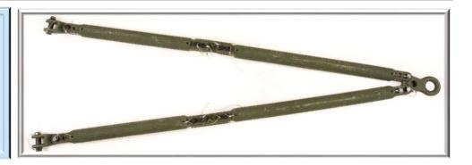
The recommended use for this tow bar is for any vehicles under (80K GVWR) that may require a longer tow bar such as the Stryker family of vehicles.
