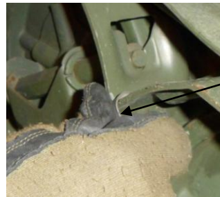
Single loop on a stationary surface, push or pull on double loop to expand single loop
